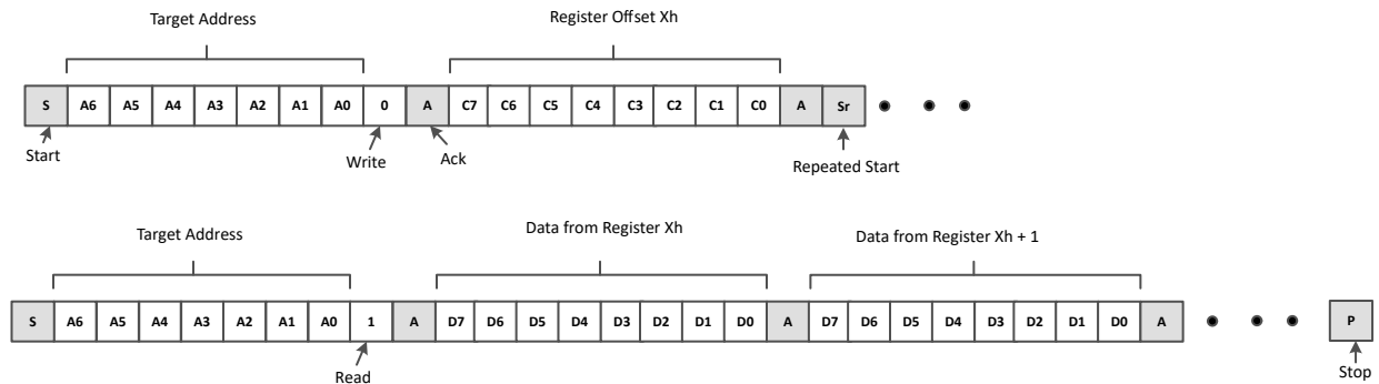
Figure 7-4. I 2 C Read with Repeated Start
