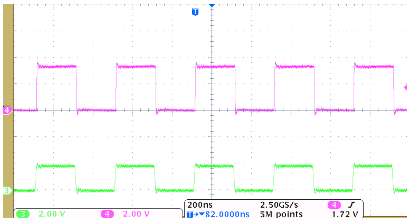
Figure 8-2. Level-Translation of a 2.5-MHz Signal
