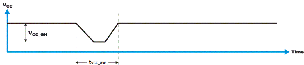
Figure 8-5. Glitch Width and Glitch Height
