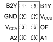
Figure 5-2. DTT Package, 8-Pin SON Transparent (Top View)
