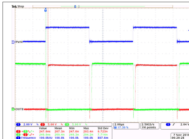
Figure 9-5. Bench Test Waveform for PWM and OUTA/B
