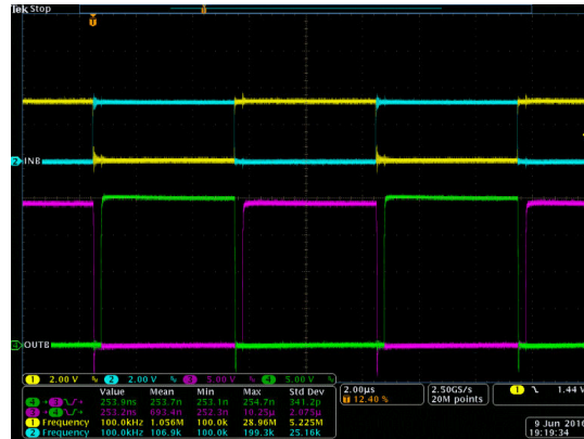
Figure 8-5. Bench Test Waveform for INA/B and OUTA/B
