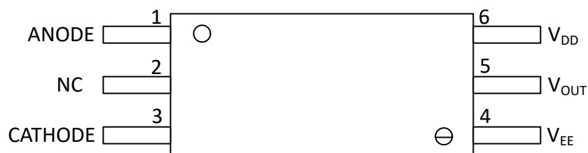
Figure 5-1. UCC23113 DWY Package SOIC-6 Top View
