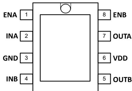
Figure 4-5. DDA Package 8-Pin SOIC Top View
