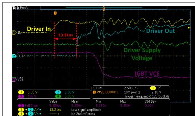
Vin = 210 V, Vout = 235 V, Iout = 1.14 A, Fsw = 125 kHz,
