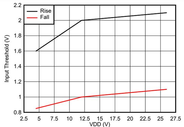
Figure 5-8. Input Thresholds
