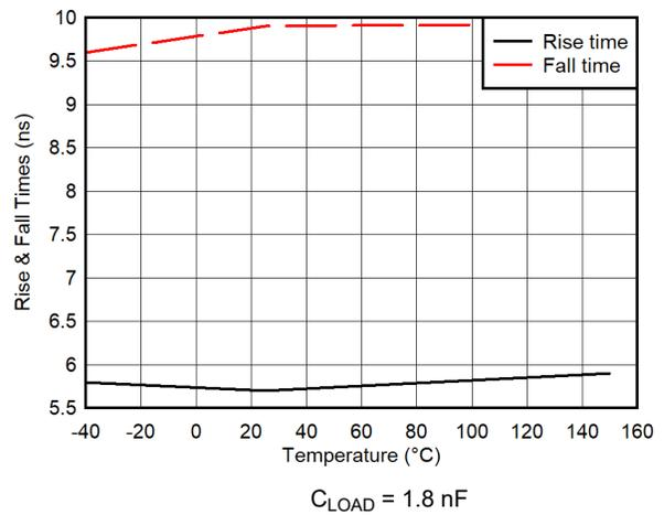
**Figure 5-16. Output Rise and Fall Time vs Temperature**
