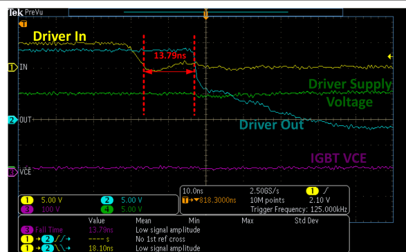
Figure 7-3. UCC27624 Used to Drive IGBT in the Boost Converter
