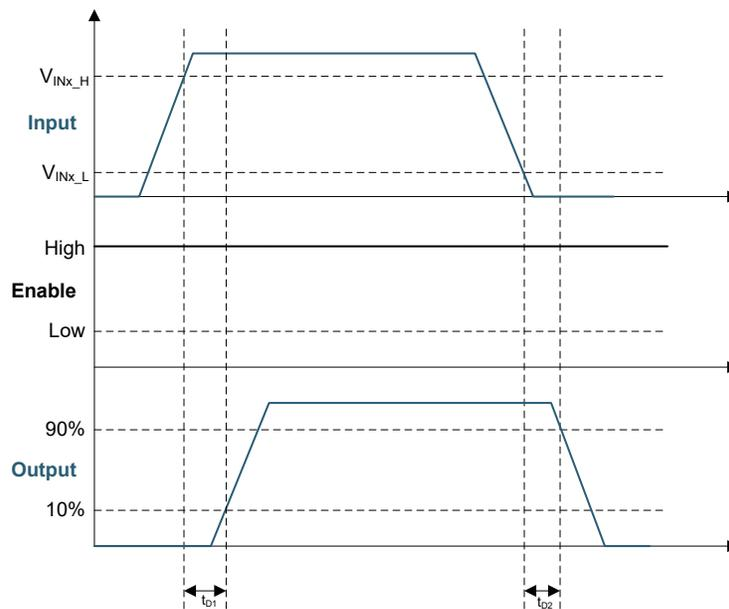
**Figure 5-2. Input-Output Operation**
