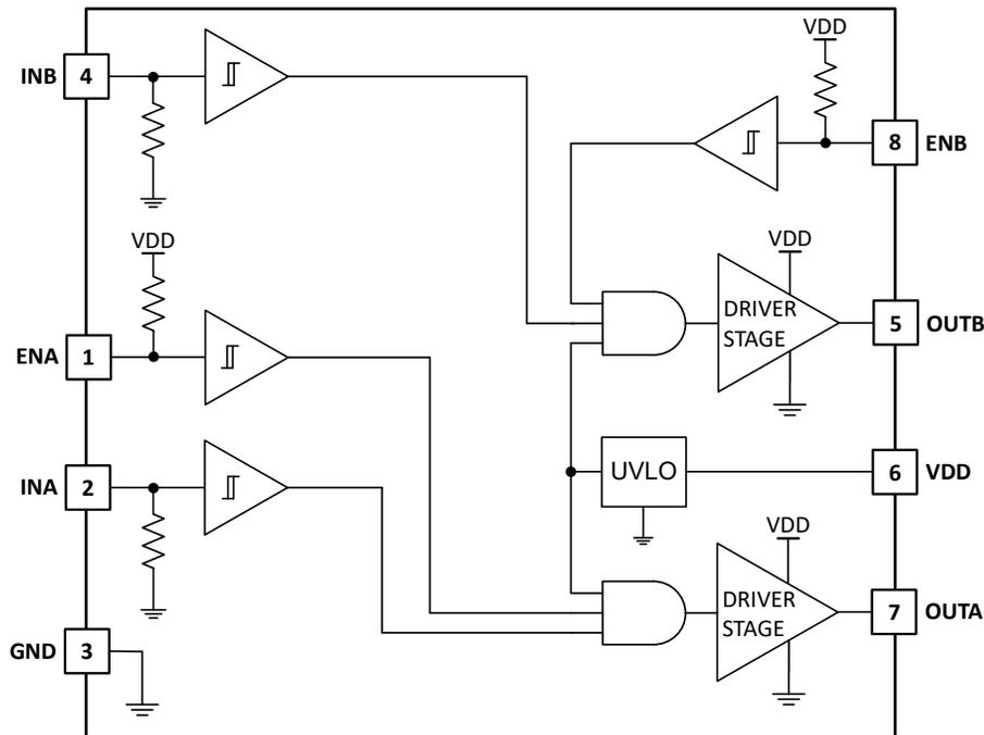
Typical ENx pullup resistance is 200 kΩ and INx pulldown resistance is 120 kΩ.
