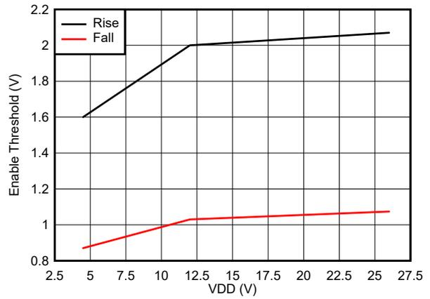
Figure 5-10. Enable Threshold
