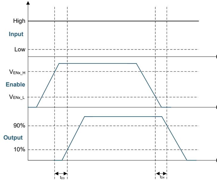
**Figure 5-1. Enable Function**
