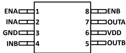
Figure 4-4. DGK Package 8-Pin VSSOP Top View
