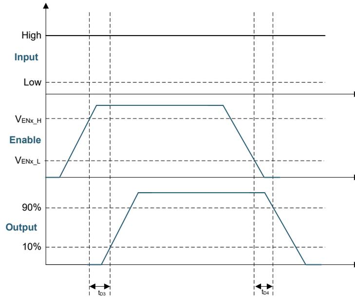
**Figure 5-1. Enable Function**
