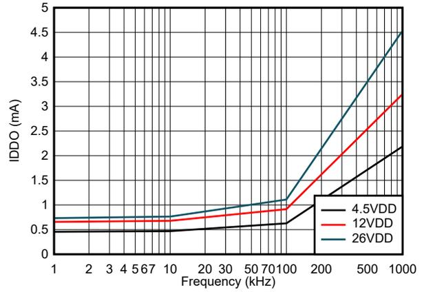
Figure 5-4. Operating Supply Current (Both Outputs Switching)
