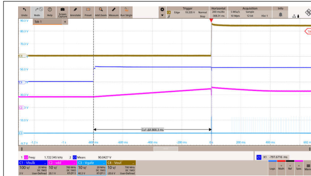
Figure 8-4. Start-Up Waveforms at 85Vac and No Load
