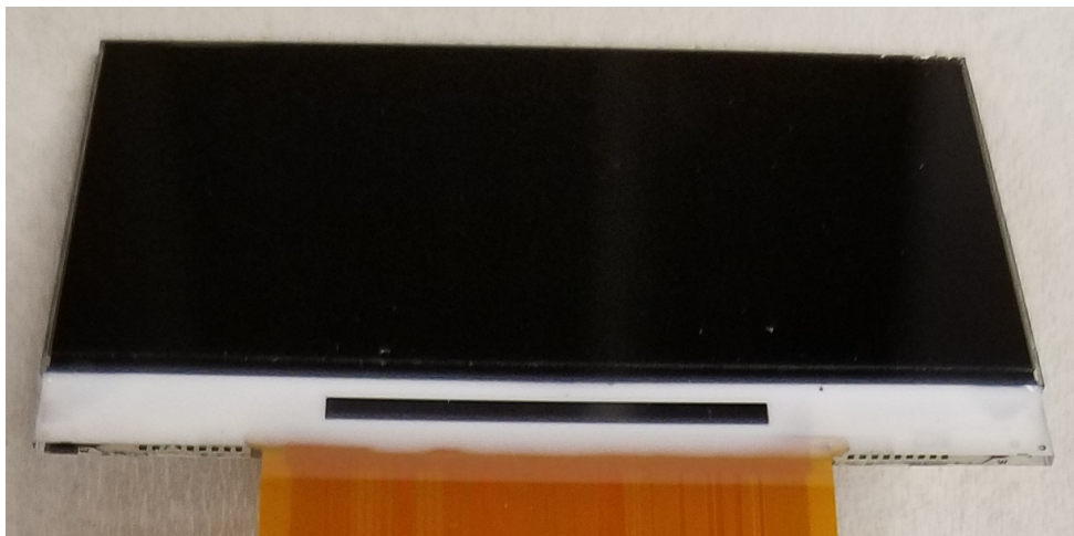
Figure 12. TFT panel used for sunlight testing. Part number E06030K16.
