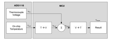
Conversion tables and polynomial equations used to determine thermocouple temperature from the thermoelectric voltage are found at the NIST website.
