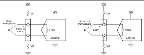
In the case of the good thermocouple, the thermocouple voltage has a range of -6.5mV to 55mV. The remaining 3.3V of the VDD supply is dropped equally between the biasing resistors. With 1-M $\Omega$  bias resistors, the thermocouple voltage has a DC operating point near mid-supply at 1.65V.
