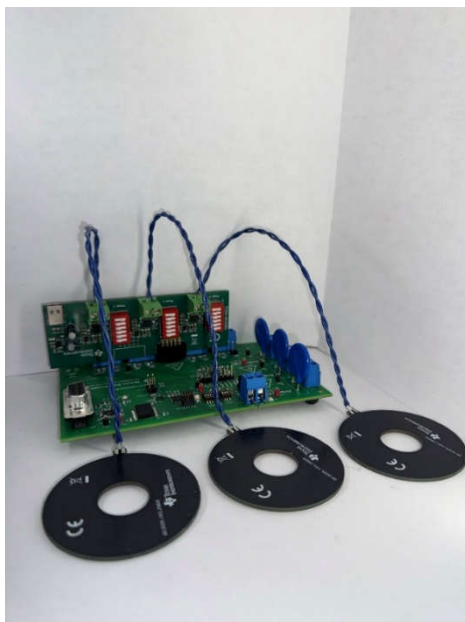
Figure 1-1. 3-phase E-meter Rogowski Coil Design with TIDA-010987, ADS131M08MET-EVM, and TIDA-010986
