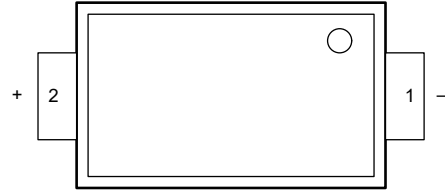
ID mark is identified as a dot in the ID area and it denotes pin 1. Figure 5-2. DYA Package 2-Pin SOT-5X3 Top View
