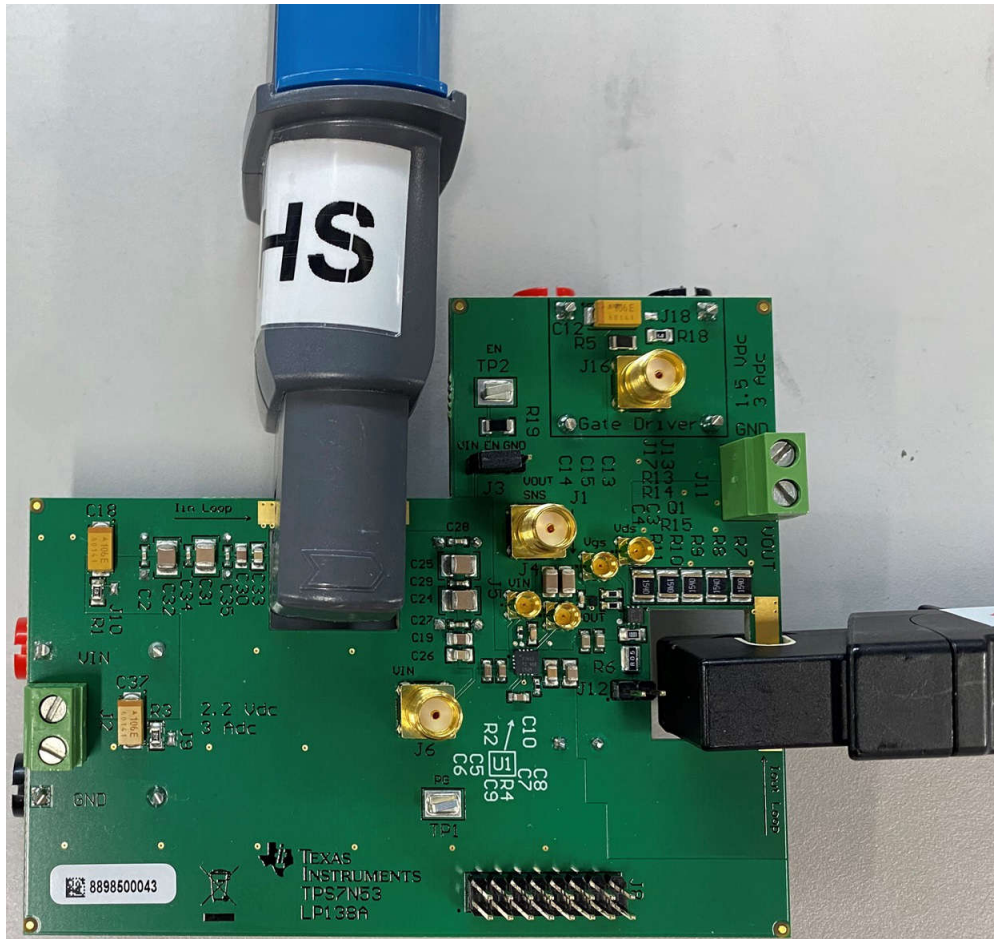
Figure 2-2. TPS7N53EVM With Current Probes Attached
