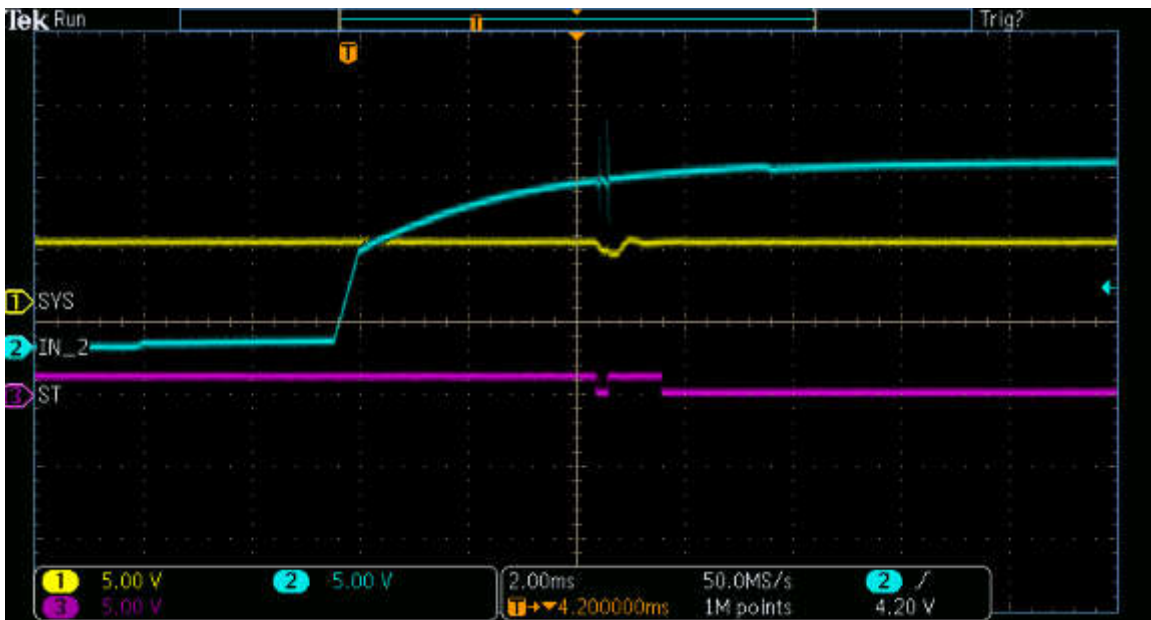
Figure 2-7. Test Five, 0uF Added Capacitance, 3A Output Current
