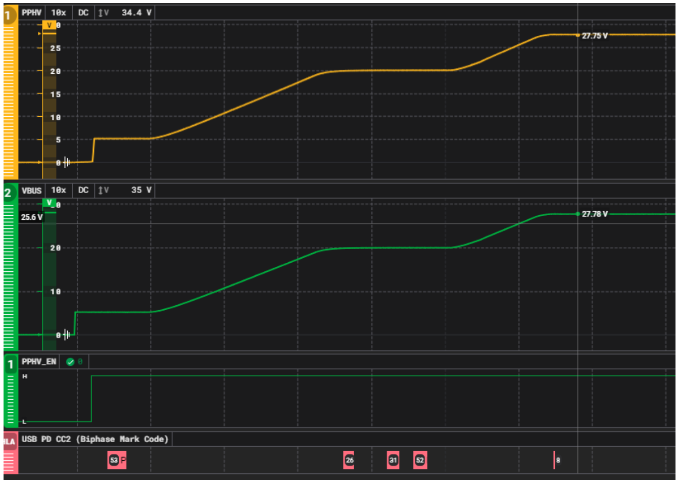
Figure 6-2. 28V USB-PD EPR Source being plugged into TPS26750
