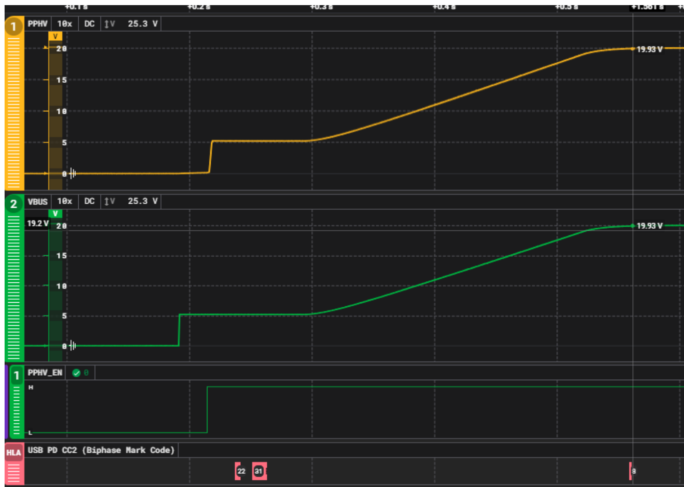
Figure 6-1. 20V USB-PD Source being plugged into TPS25751
