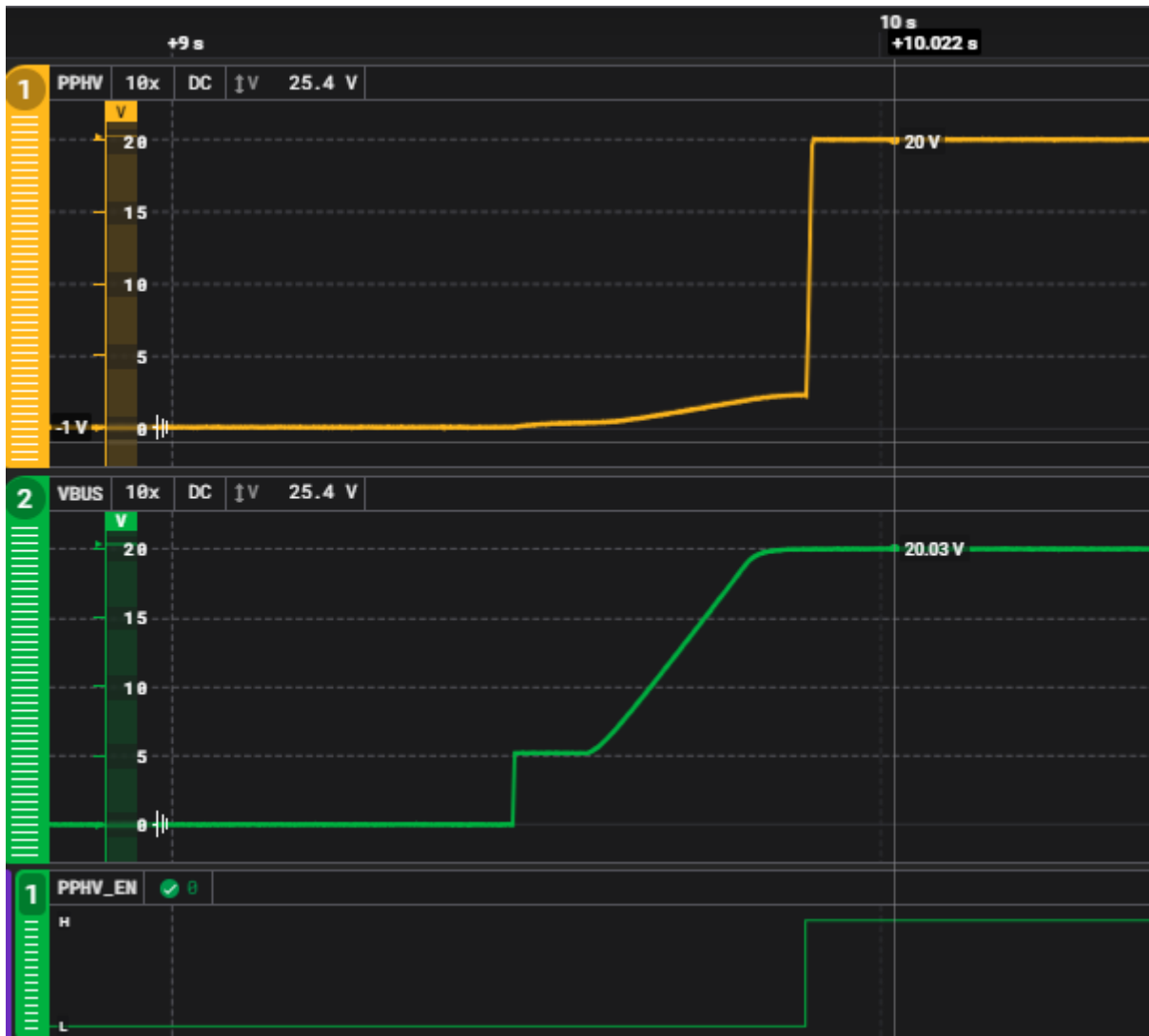
Figure 3-7. Capability Mismatch is not asserted in the Request Message
