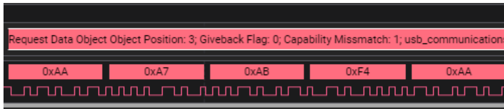
Figure 3-4. Request Data Object from the PD Device to the PD Source
