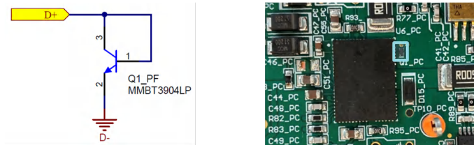
Figure 3-5. Small and Cost Effective Implementation of Temperature Monitor with a BJT in Diode Configuration in Close Proximity to Each of the TPS7H6101-SEP Power Stage Devices
