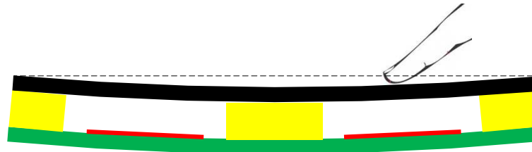
Figure 21. Mechanical Structure Is Not Rigid Enough
