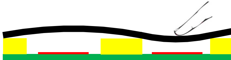
Figure 20. Issue Due to Elastic Adhesive
