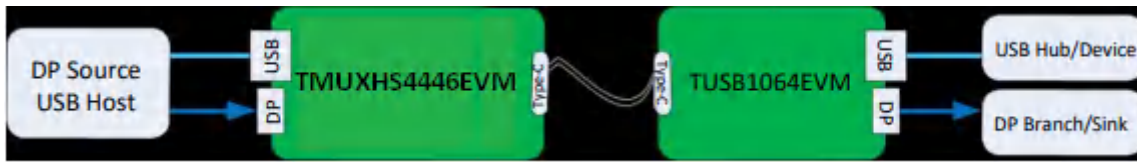
Figure 1-1. TMUXHS4446EVM Typical Test Setup
