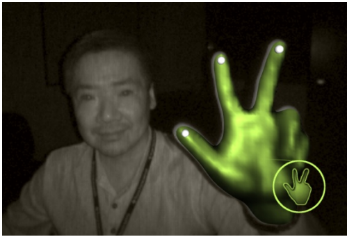
Figure 11: Gesture recognition using a 3D-TOF sensor and SoftKinetic iisu® middleware.
