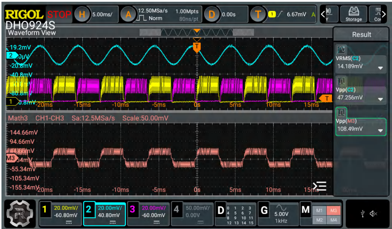
Figure 4-7. 200Hz Input at 75% Volume – High PWM Activity
