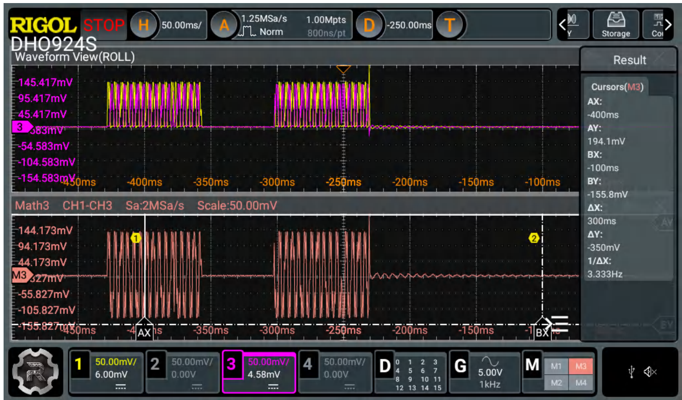
Figure 2-1. Open-Loop LRA Waveform for Double-Click Effect
