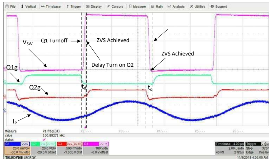
Figure 6. V_{IN} = 380\text{ V} , I_{OUT} = 10\text{ A} , ZVS at f_r
