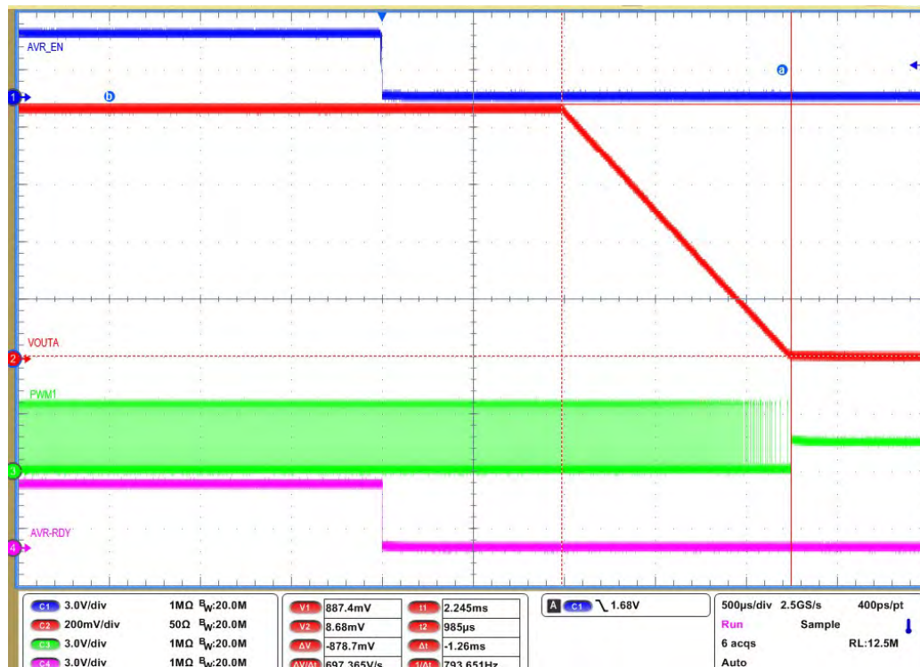
Figure 6-4. VOUTA Enable OFF Soft-off with TOFF delay=1ms
