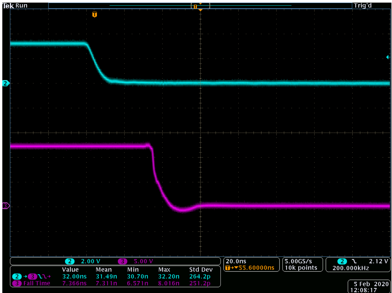
Figure 5. Example Input and Output Waveforms, Zoom In on Fall (Input: Ch2, Output Ch3)
