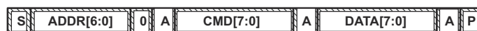
Figure 4-2. Attempt To Write a Read-Only Address (Nack After Data Sent By Controller)
