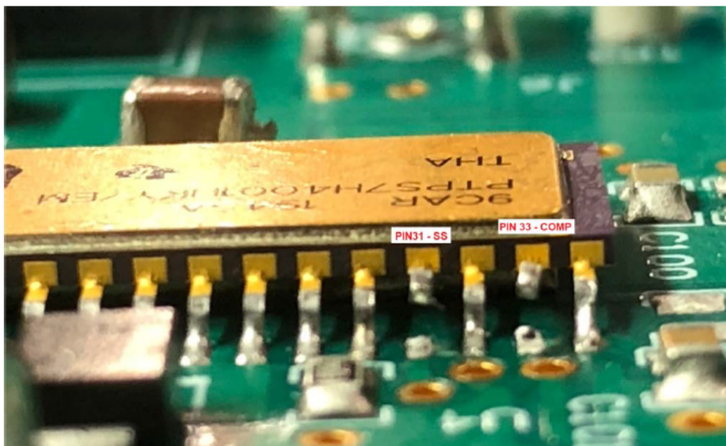
Figure 6. Lift Pins 2, 31, 33 from PCB
