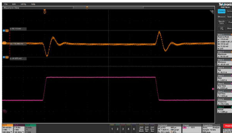
Figure 3-1. TPS54JB20 Transient Response with D-CAP3
