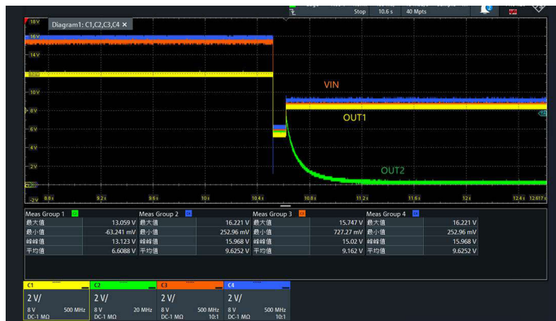
Figure 3-2. Output Channel 2 (No Load) Latch-off After the Input Voltage Drops and Recovers
