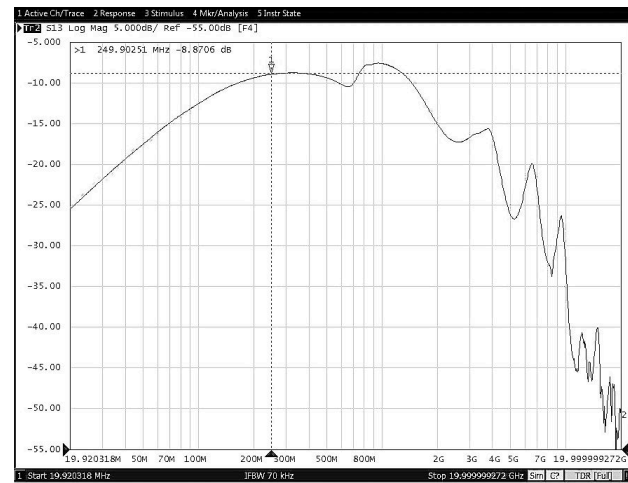
Figure 8-30. Off-State Data-Switch Isolation vs Frequency (TPS25830A-Q1)
