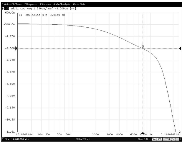
Figure 8-29. Data Transmission Characteristics vs Frequency (TPS25830A-Q1)
