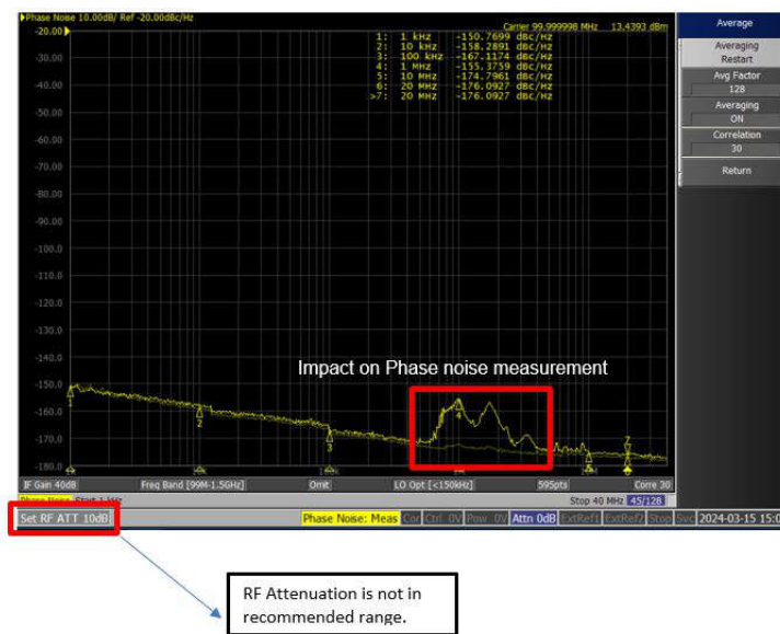
Figure 3. 5052B Settings impact on phase noise
