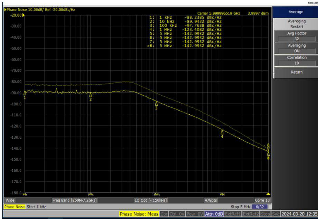
Figure 8. 6GHz output on LMX2820 with reference (OSCIN) levels of -5dbm and 10dbm
