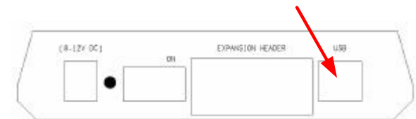
Figure 5. ADC08(B)3000RB rear panel showing location of USB connector
