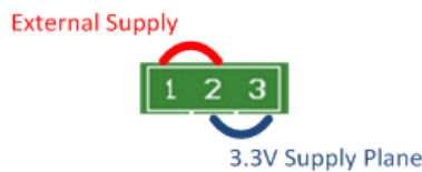
Figure 4-4. J13, J16, J20 Connection Description
