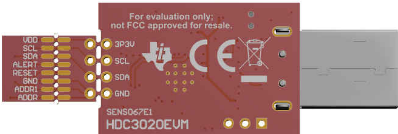
Figure 3-5. Bottom Layer of the HDC3020EVM
