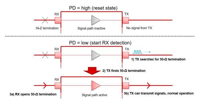
Figure 4-1. Redriver RX Detection Functionality
