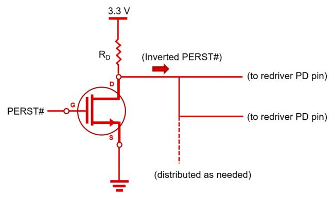
Figure 4-2. Inverted PERST# Distribution Example to Redriver PD Pins
