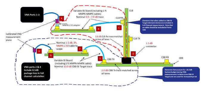
Figure 2-8. PCI-SIG System RX Calibration Specifications
