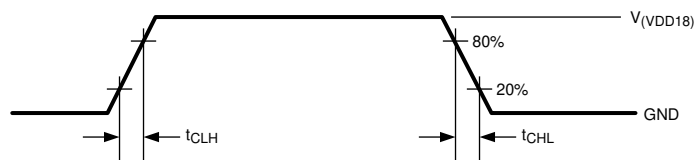
Figure 5-1. LVC MOS Transition Times
