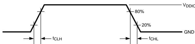
Figure 3. LVCMOS Transition Times
