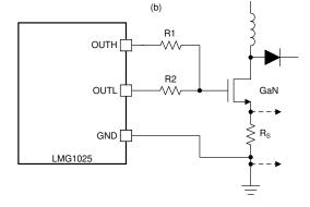
Figure 7-2. Source Resistor Current Sense A Configuration
