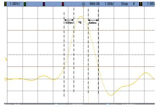
Figure 7-8. Input Pulse Width and Propagation Delays
