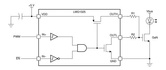
Figure 7-1. Typical Implementation of a Circuit
