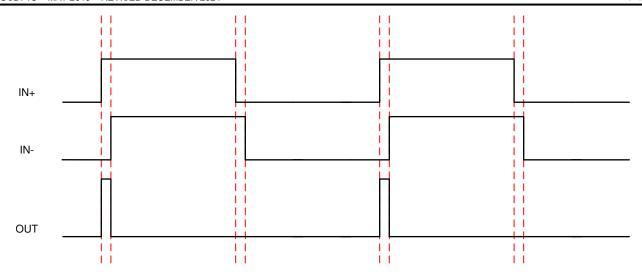
Figure 7-5. Timing Diagram To Create Short Pulses
