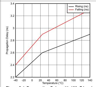
Figure 5-4. Propagation Delay with 100pF Load
