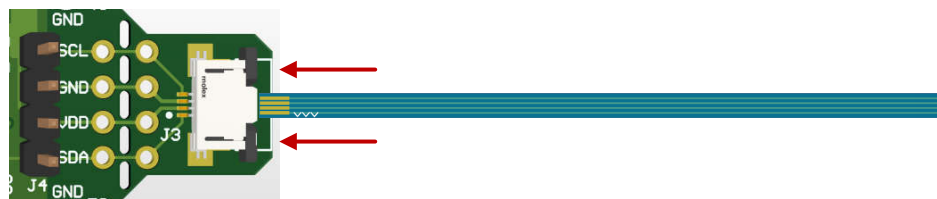
Figure 2-3. Inserting FPC Board and Locking Connector
