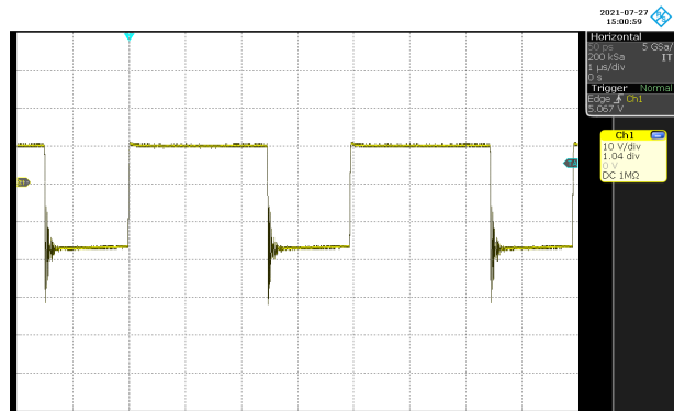
Figure 6-9. PIV of D7 (main Output Rectifier) Under 100% Load and 16-V Maximum V_{IN}
