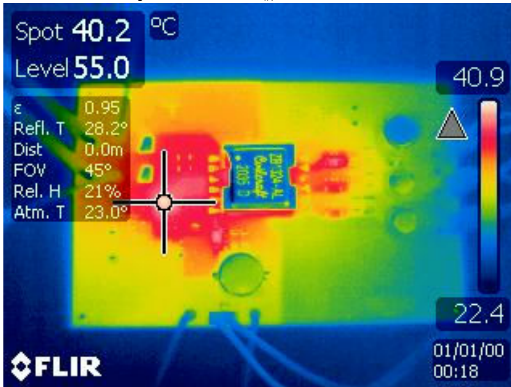
Figure 6-25. EVM Thermal Image at 12 V IN and 100% Load
