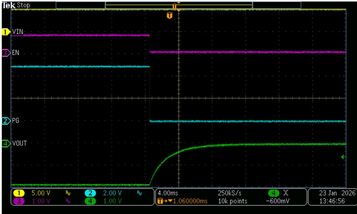
**Figure 3-7. Power Good De-assert - EN Independently Driven LOW**
