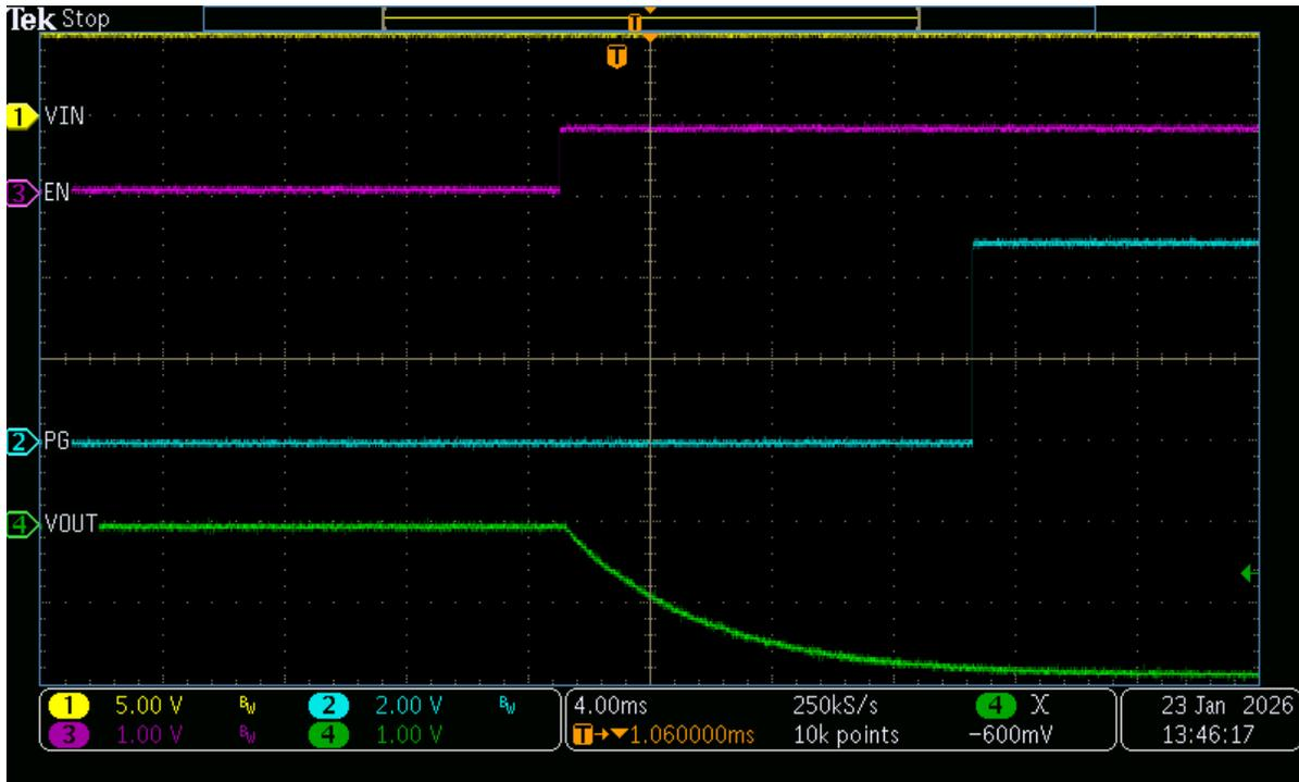
**Figure 3-3. Power Good Assert - EN Independently Driven HIGH**
