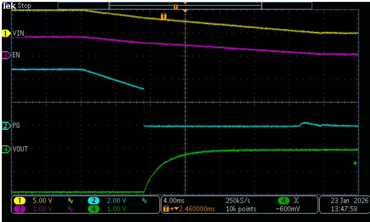
**Figure 3-8. Power Good De-assert - EN Tied to Falling VIN via Resistor Divider**
