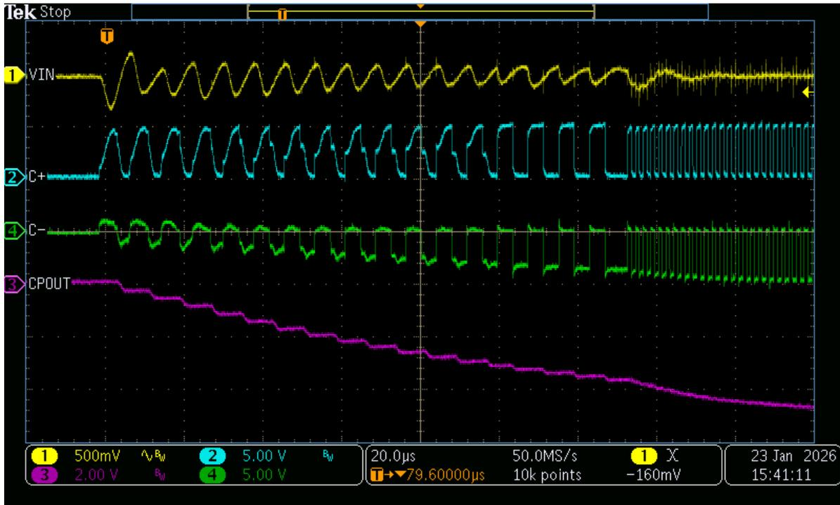
Figure 3-10. VIN Ripple
