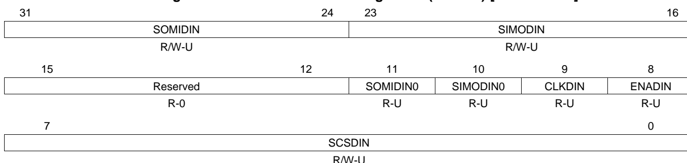
Figure 21-24. SPI Pin Control Register 2 (SPIPC2) [offset = 1Ch]
