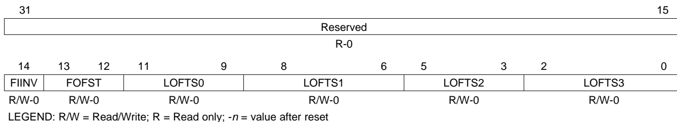
Figure 10-29. External Memory Line Offset Register (SDOFST)
