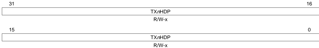
Figure 6-70. Transmit Channel n DMA Head Descriptor Pointer Register (TX n HDP)
