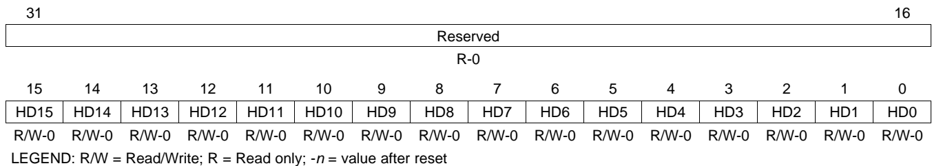
Figure 20-21. GPIO Data 1 Register (GPIO_DAT1)
