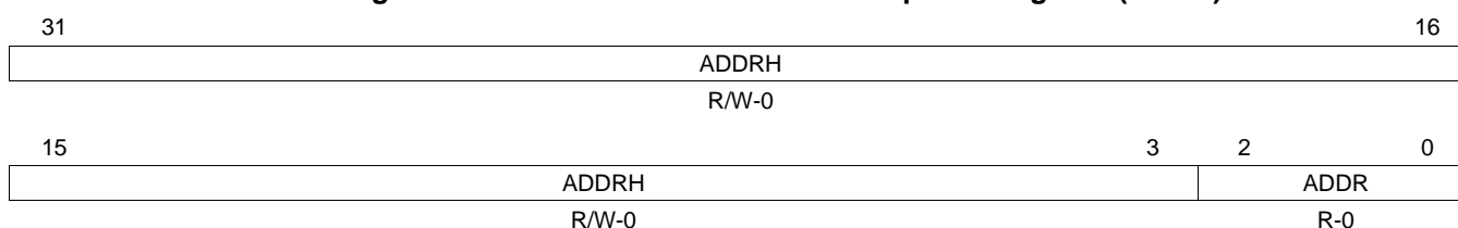
Figure 31-28. uPP DMA Channel I Descriptor 0 Register (UPID0)
