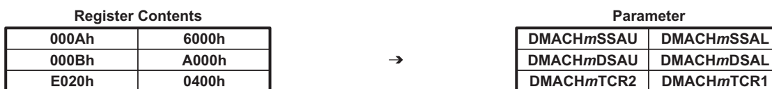
Figure 3-7. Block Move Example DMA Configuration
