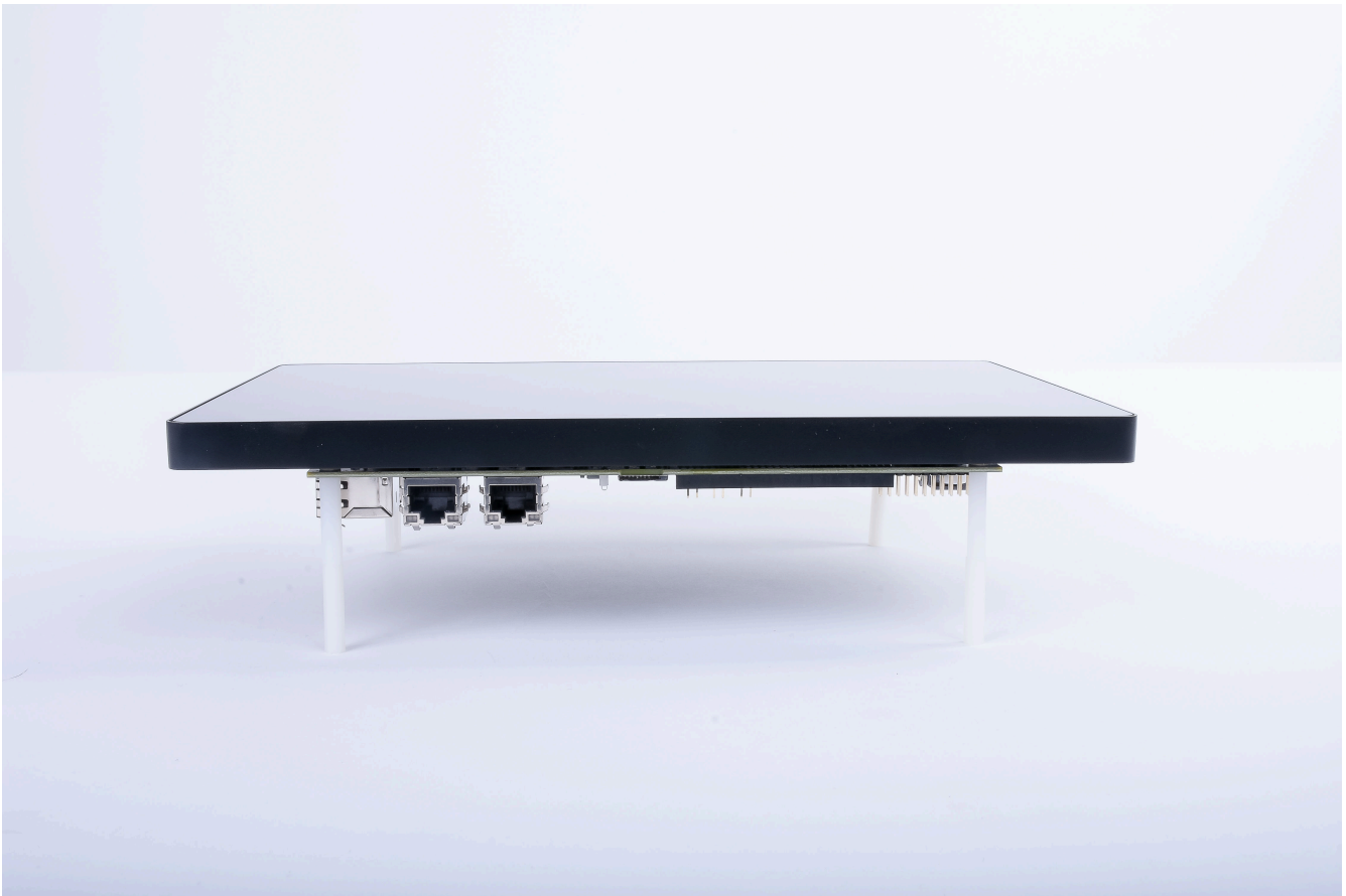
Figure 2-3. AM572x IDK EVM with LCD Display Assembly Attached - Top View
