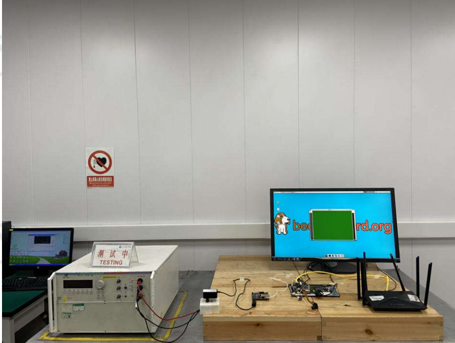
SURGES TEST SETUP
