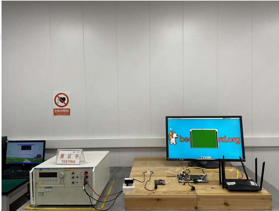
SURGES TEST SETUP
