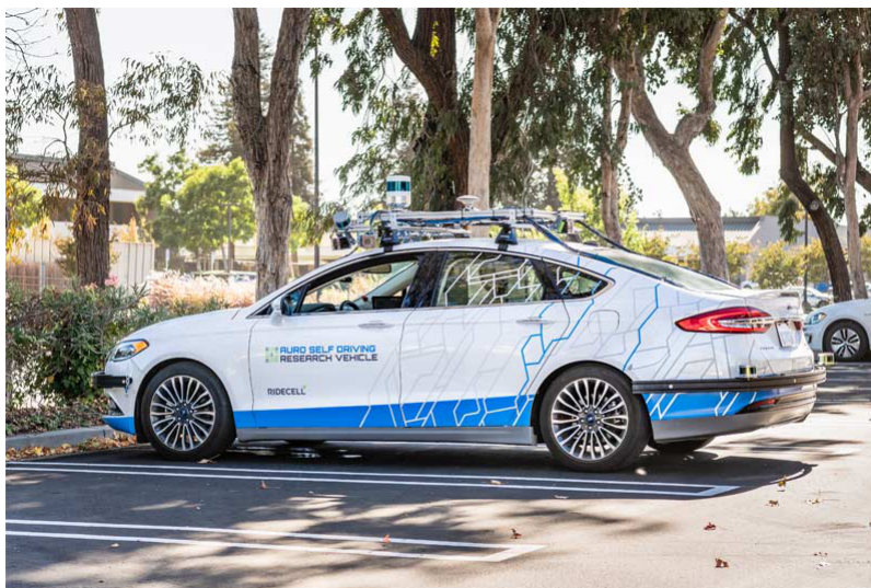
Figure 2. An Autonomous Vehicle Equipped with Lidar
