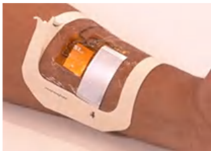
Figure 2. Use flex PCB designs with strong adhesive coverings or backings to avoid lifting the sensor away from the skin
